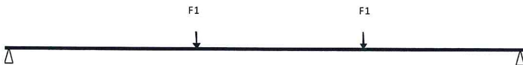
Figure Q5. A simply supported beam at both ends carrying two point loads
