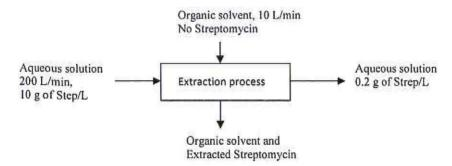
Figure 4.1. Extraction process of Streptomycin from aqueous solution.
