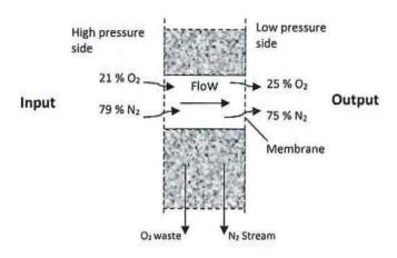
Figure 5.1. Separation of oxygen and nitrogen using a membrane.
